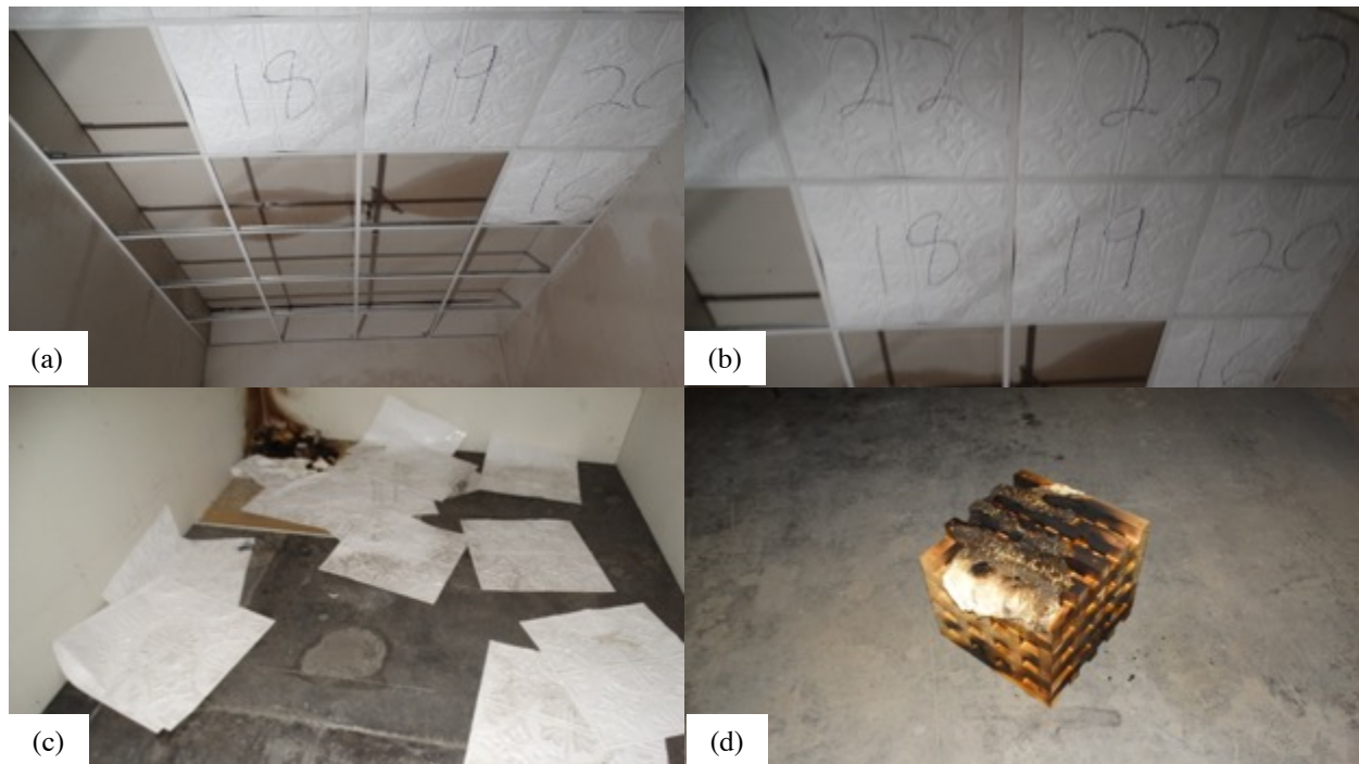
Figure 7. Test 1 post-test images showing (a-b) remaining ceiling tiles, (c) fallen tiles, and (d) removed crib.
